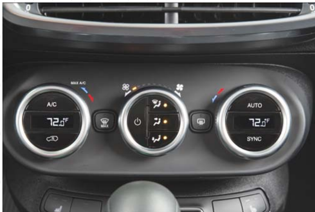
Automatic Temperature Controls (ATC)
