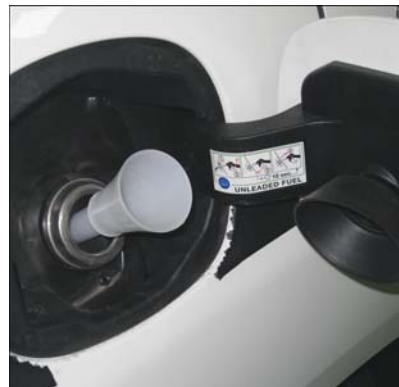
Emergency Fuel Filling Procedure
