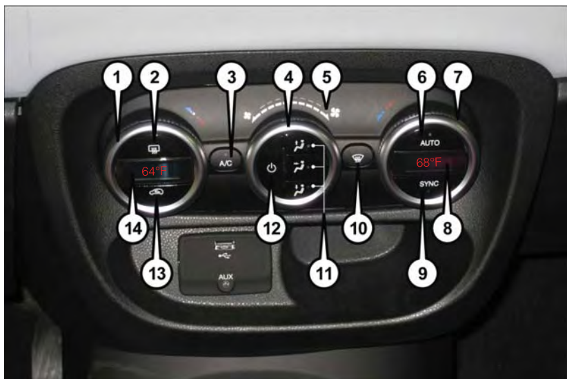
Automatic Temperature Controls (ATC)
