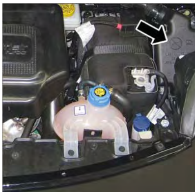
Front Distribution Unit
