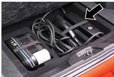
EVSE Rear Cargo Location
