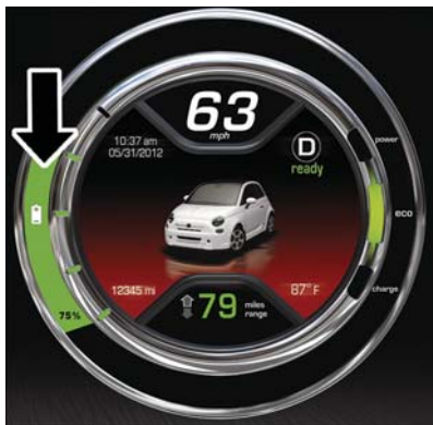
High Voltage Battery Gauge
