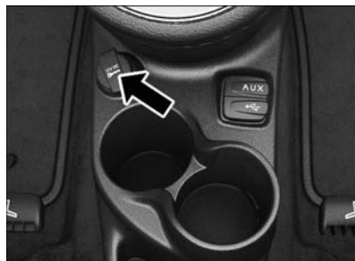
Center Stack Power Outlet
