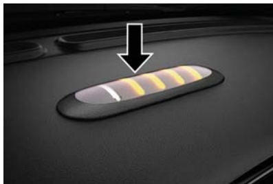
State Of Charge Indicator
