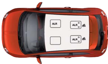
ALR — Switchable Automatic Locking Retractor
