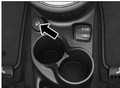
Center Stack Power Outlet
