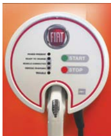
Electric Vehicle Supply Equipment (EVSE)
