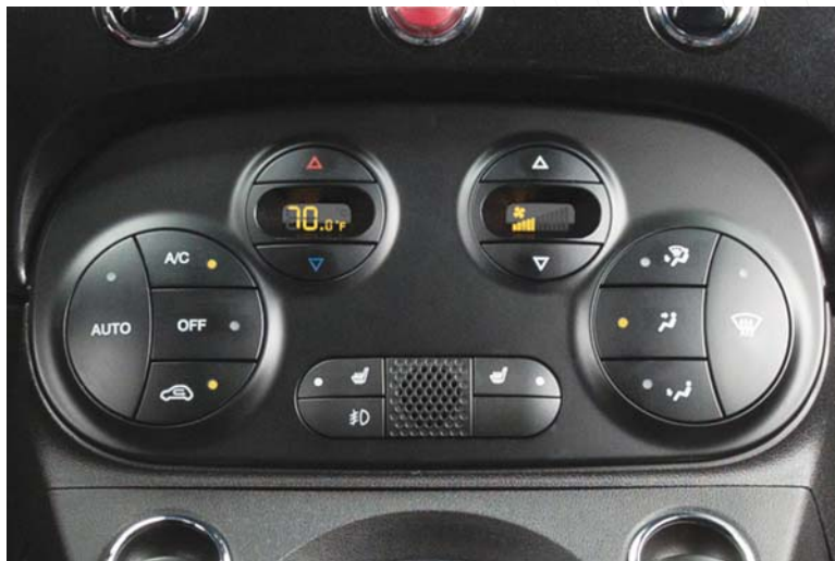
Automatic Temperature Controls
