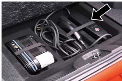
EVSE Rear Cargo Location
