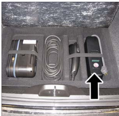
Electric Vehicle Supply Equipment (EVSE)
