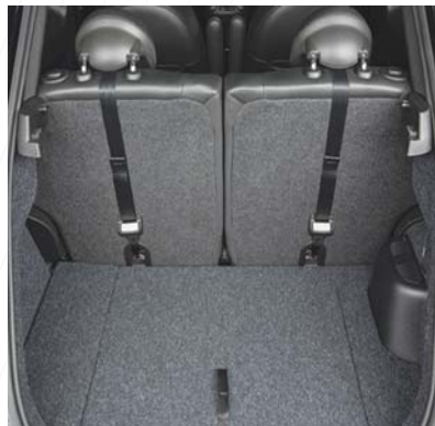
Rear Seat Tether Strap Mounting
