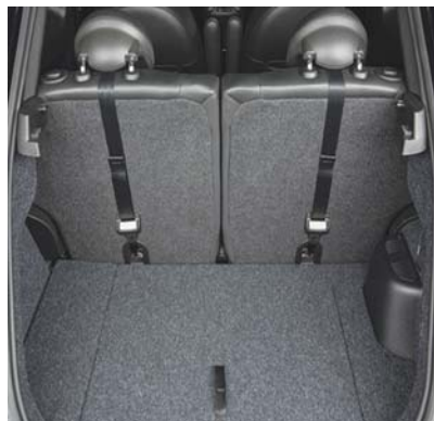
Rear Seat Tether Strap Mounting
