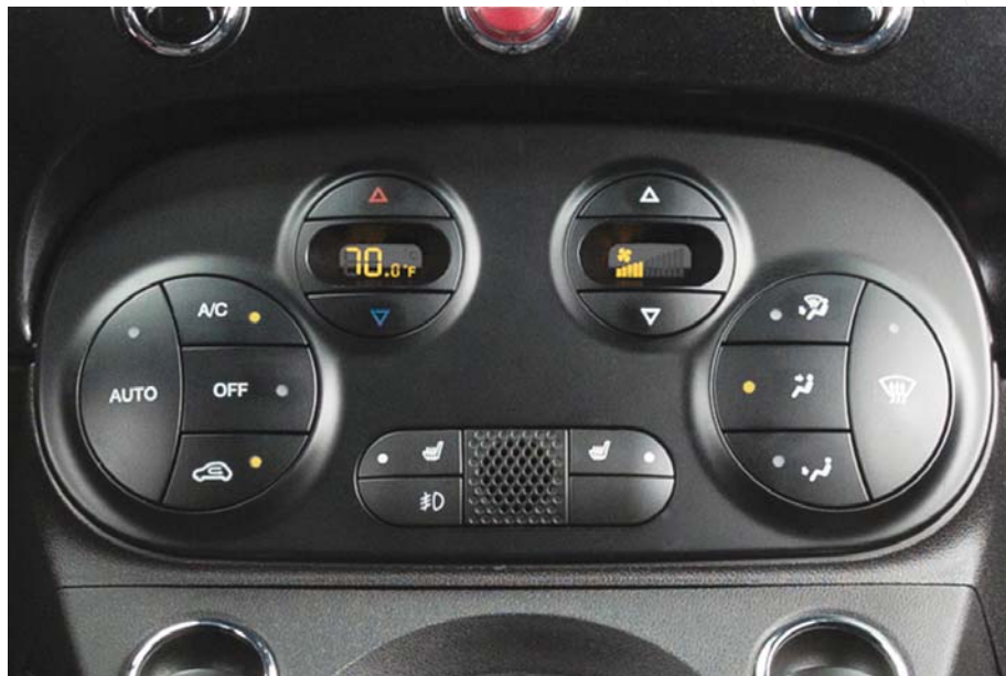
Automatic Temperature Controls
