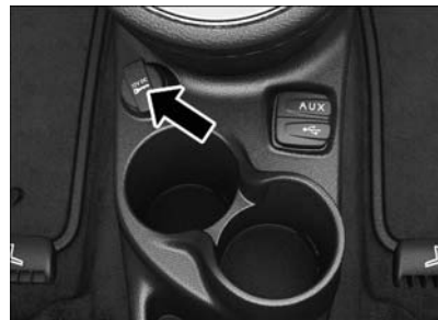
Center Stack Power Outlet
