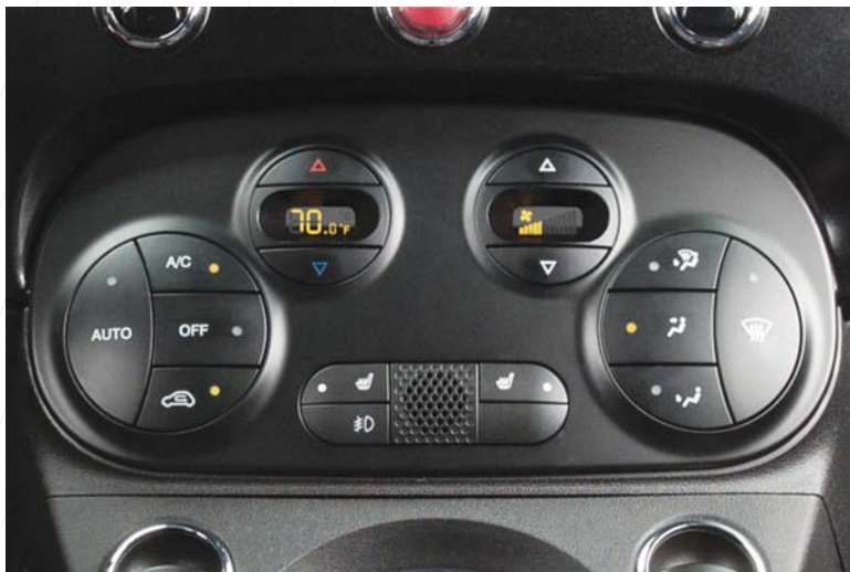
Automatic Temperature Controls
