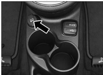
Center Stack Power Outlet
