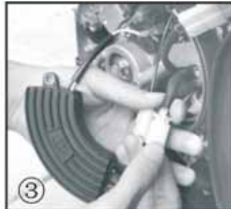
③ Disconnect the wire clip.
