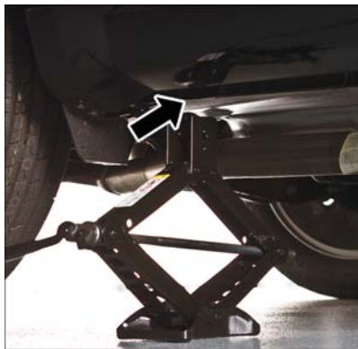
Front Jacking Location
