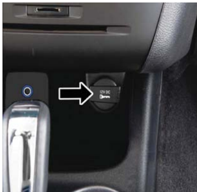
Front Power Outlet
