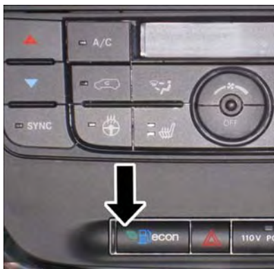
ECON Switch Location
