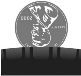
Exposed tread bars (replace)
