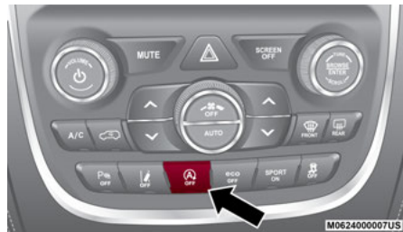
STOP/START Off Switch
