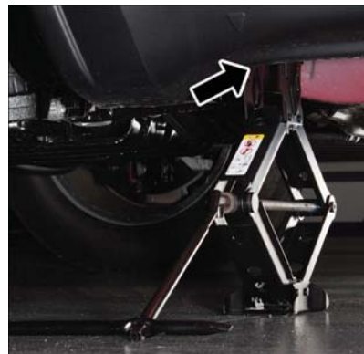
Front Jacking Location
