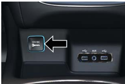
Front Power Outlet
