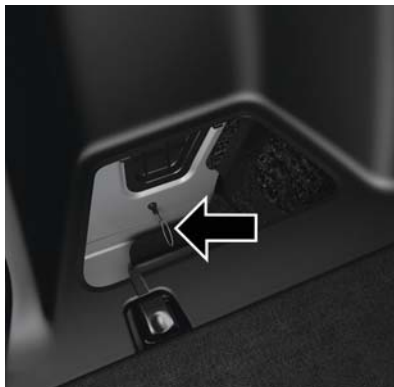
Emergency Release Cable
