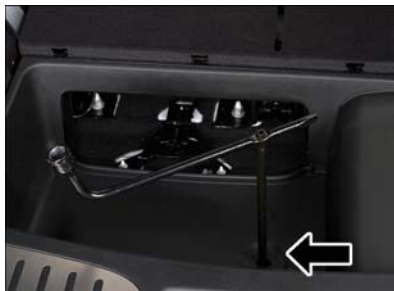
Winch Drive Nut Location
