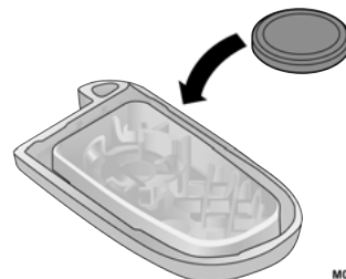
Key Fob Battery Replacement
