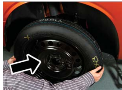
Installing Compact Spare
