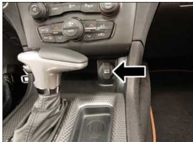
Front Power Outlet
