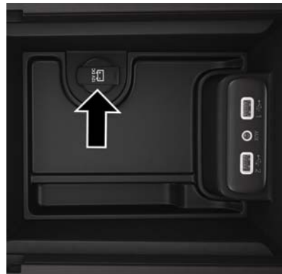
Center Console Power Outlet
