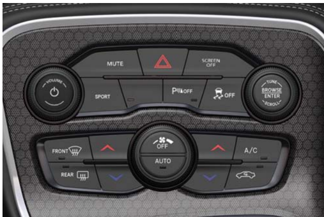
Automatic Climate Controls On The Faceplate
