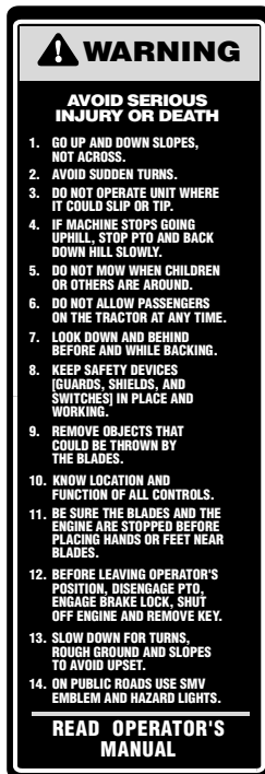
INSTRUCTION / WARNING LABEL ON LEFT RUNNING BOARD
