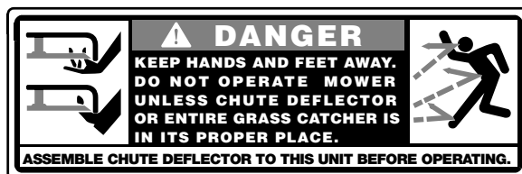
DEFLECTOR AND SAFETY LABEL LOCATED ON RIGHT SIDE OF DECK
