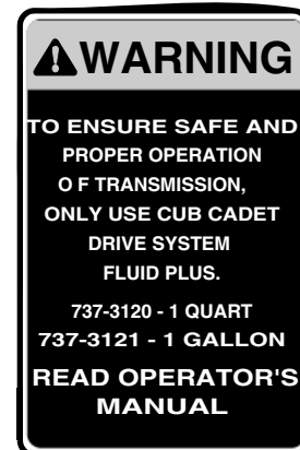
TRANSMISSION OIL GRAPHIC ON REAR HITCH PLATE
