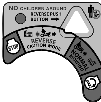
KEY SWITCH/MODULE GRAPHIC– LOCATED ON DASH PANEL
