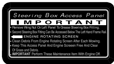
STEERING GEAR/ENGINE SCREEN MAINTENANCE–ON LH ENGINE SHIELD AT FRONT OF DASH PANEL
