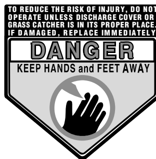
HANDS/FEET SAFETY GRAPHIC - ON DECK DEFLECTOR CHUTE
