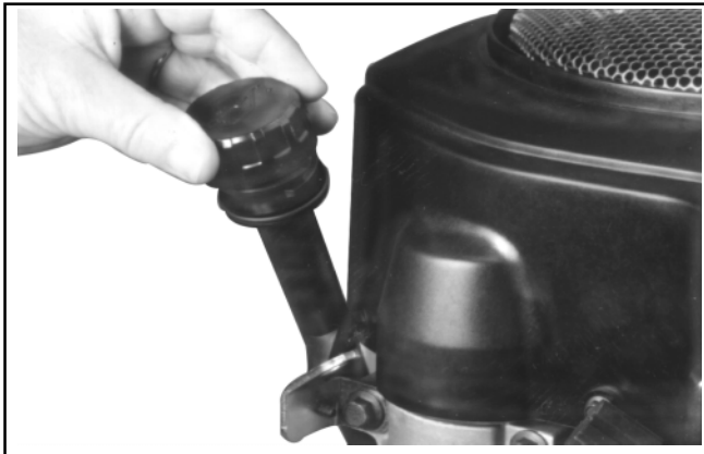
Figure 6. Checking Oil Level.
