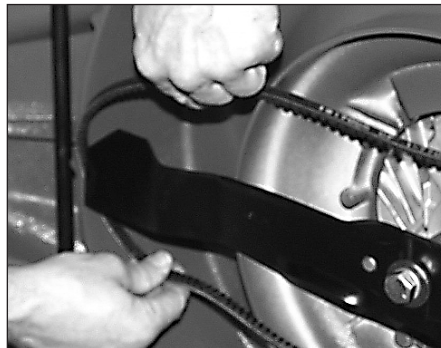
Figure 5-8: Remove or install belt around blade.
