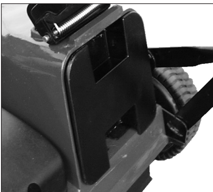
Figure 4-4: Installed Mulching Plug.
