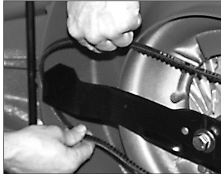
Figure 5-8: Remove or install belt around blade.
