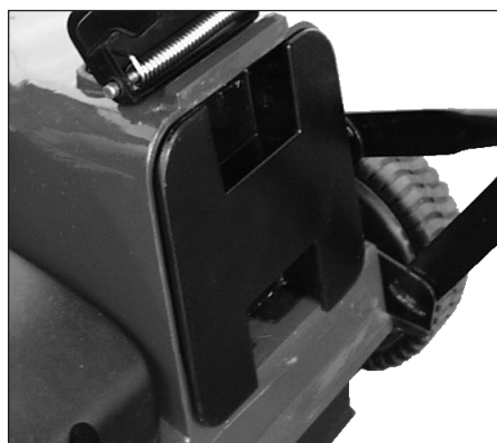
Figure 4-4: Installed Mulching Plug.
