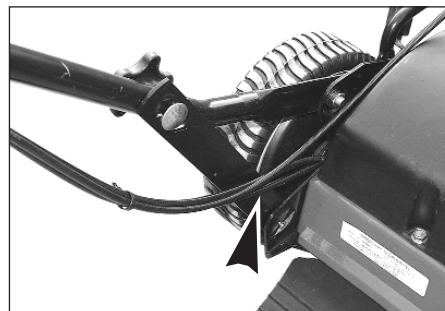
Figure 2-4: Cables correctly routed inside handlebar strut.
