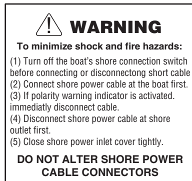
Shore Power Connection
