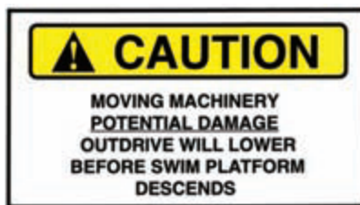
Above Hydraulic Swim Platform Switch
