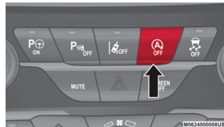
Stop/Start OFF Switch
