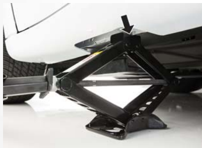
Front Jacking Location Engaged
