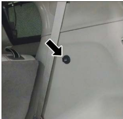
Rear Power Outlet
