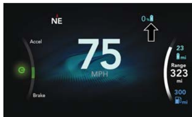
High Voltage Battery Gauge
