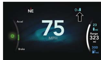
High Voltage Battery Gauge
