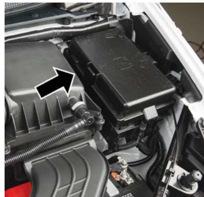
Power Distribution Center
