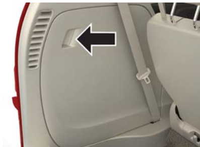
Jacking Equipment Location
