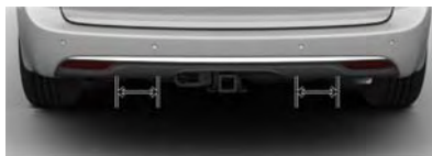
Hands-Free Liftgate Trailer Tow Activation Zones
