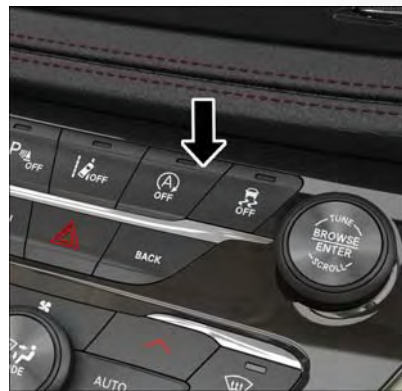
STOP/START Off Switch
