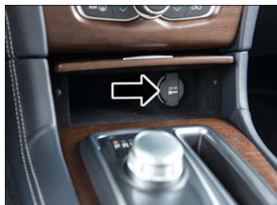
Front Power Outlet
