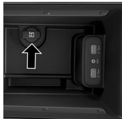
Center Console Power Outlet
