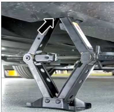
Front Jacking Location Engaged
