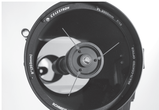
Secondary Mirror Collimation Adjustment Screws
