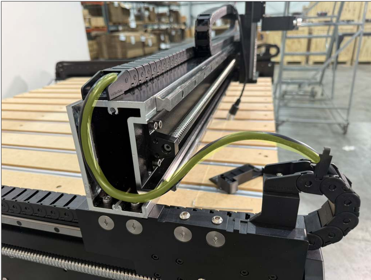
install lower spindle drag chain
