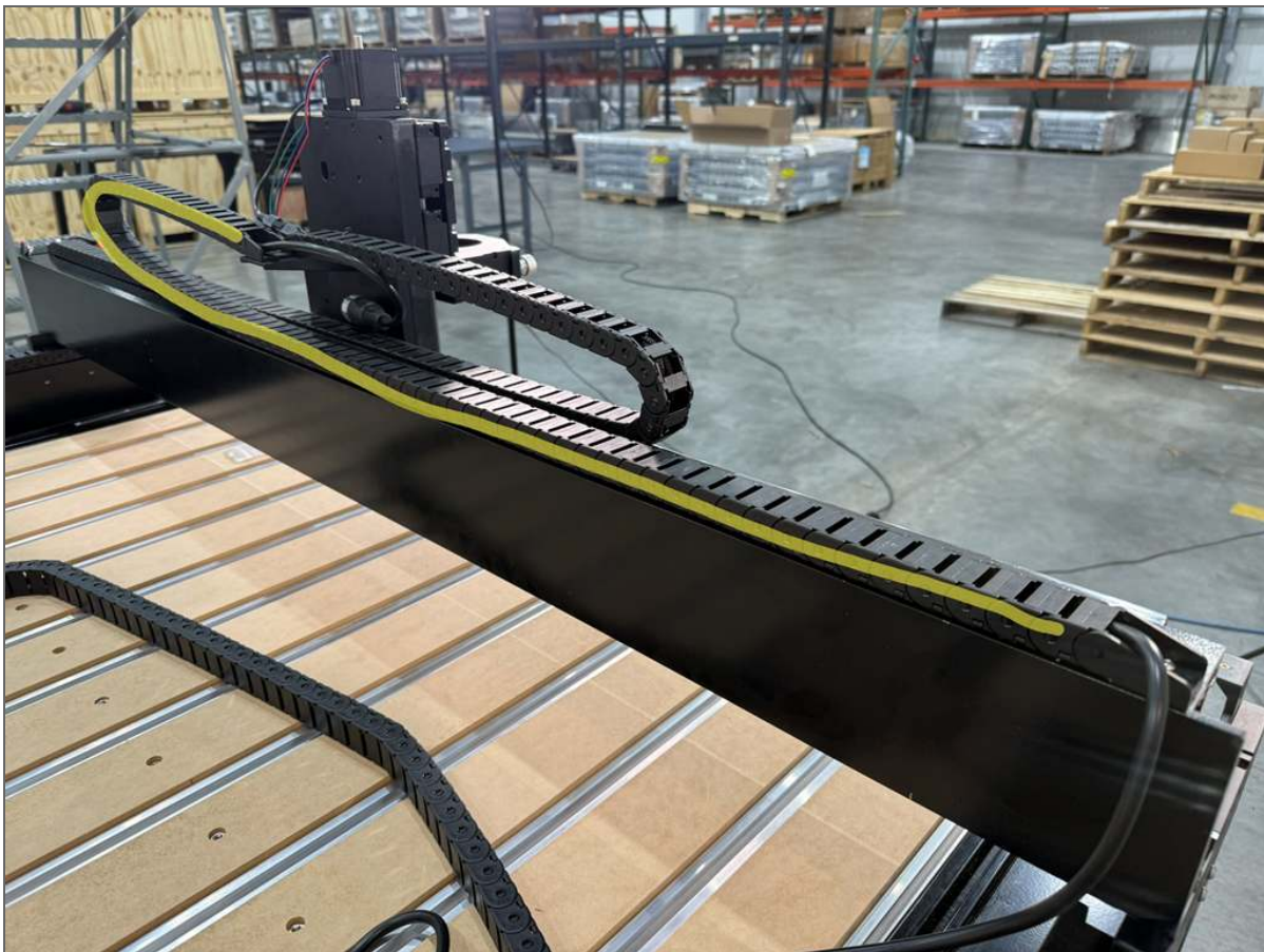
install upper spindle drag chain
