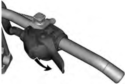
Thumb accelerator position : push downward to rotate accelerator housing
