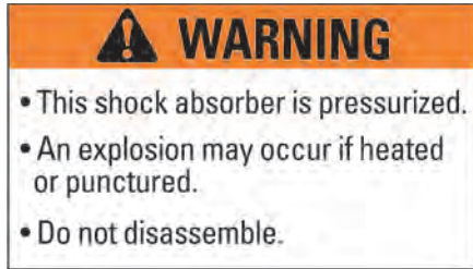
shock absorbers - Warning Label
