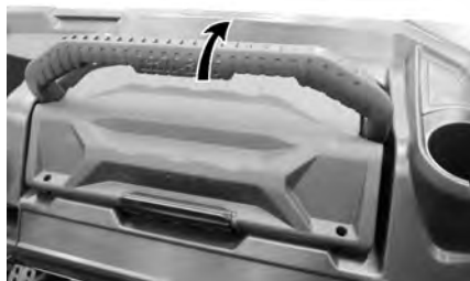
SECURING TOOL BOX IN PLACE
