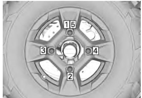
TIGHTENING SEQUENCE
