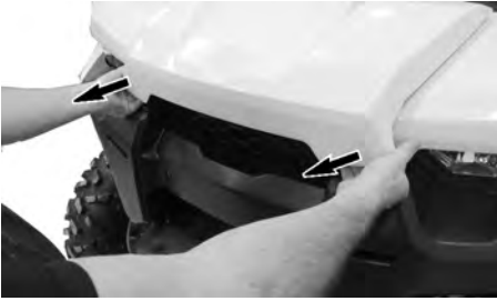
PULLING ON FRONT SERVICE COVER EDGE.
