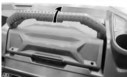
SECURING TOOL BOX IN PLACE
