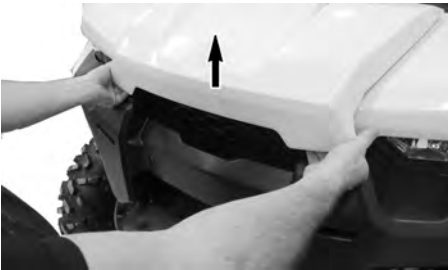
LIFTING FRONT SERVICE COVER EDGE.
