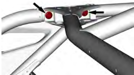
REAR LATERAL FASTENERS - TYPICAL
