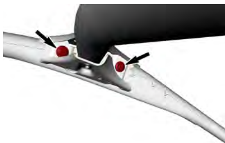
FRONT LATERAL FASTENERS - TYPICAL
