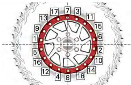
TYPICAL - TIGHTENING SEQUENCE
