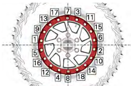
TYPICAL - TIGHTENING SEQUENCE
