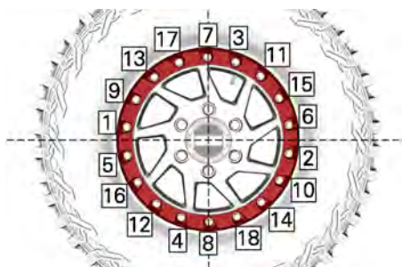
TYPICAL - TIGHTENING SEQUENCE
