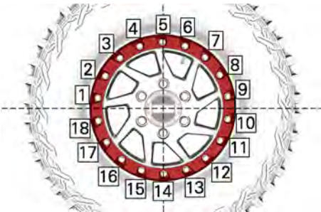
TYPICAL - FINAL TIGHTENING SEQUENCE
