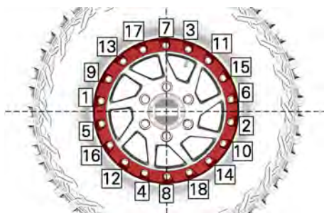
TYPICAL - TIGHTENING SEQUENCE
