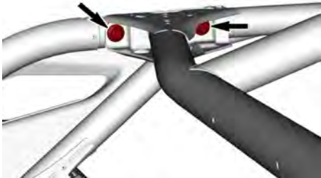
REAR LATERAL FASTENERS - TYPICAL
