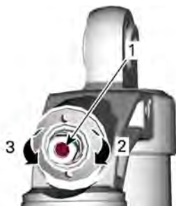
LOW-SPEED COMPRESSION DAMPING (USE A SCREWDRIVER)
