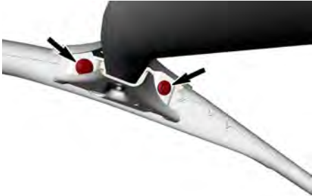
FRONT LATERAL FASTENERS - TYPICAL
