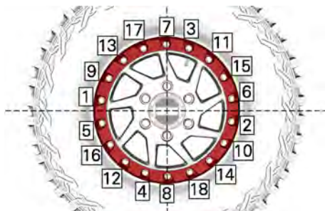
TYPICAL - TIGHTENING SEQUENCE
