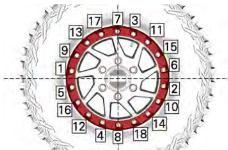
TYPICAL - TIGHTENING SEQUENCE
