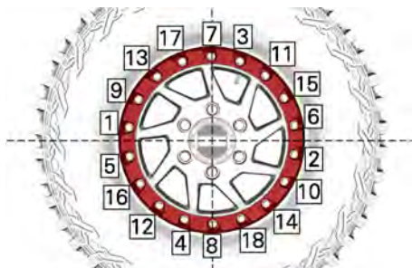
TYPICAL - TIGHTENING SEQUENCE
