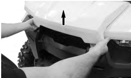
LIFTING FRONT SERVICE COVER EDGE.
