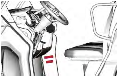
TYPICAL - NRMM IDENTIFICATION LABEL
