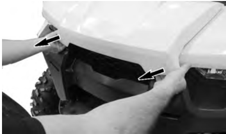
PULLING ON FRONT SERVICE COVER EDGE.
