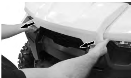
PULLING ON FRONT SERVICE COVER EDGE.
