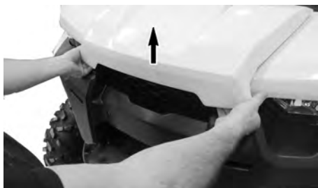
LIFTING FRONT SERVICE COVER EDGE.
