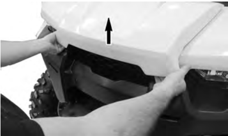
LIFTING FRONT SERVICE COVER EDGE.
