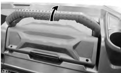
SECURING TOOL BOX IN PLACE
