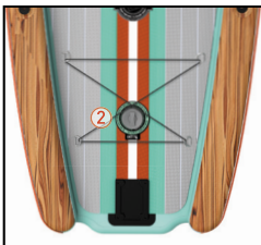
Chamber 3 - Aero Paddle Seat Bottom: 7-10 PSI Max
