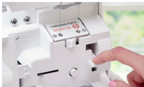
Jet-Air Threading™ With just the touch of a lever, thread is sent through the tubular loopers. There are no thread guides, no struggling and there's plenty of time to serge away!
