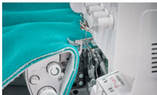
Advanced Knife Driving & One-Way Clutch System Baby Lock has created a knife system with a larger cutting bite that cuts thicker fabric with ease and increased visibility.
